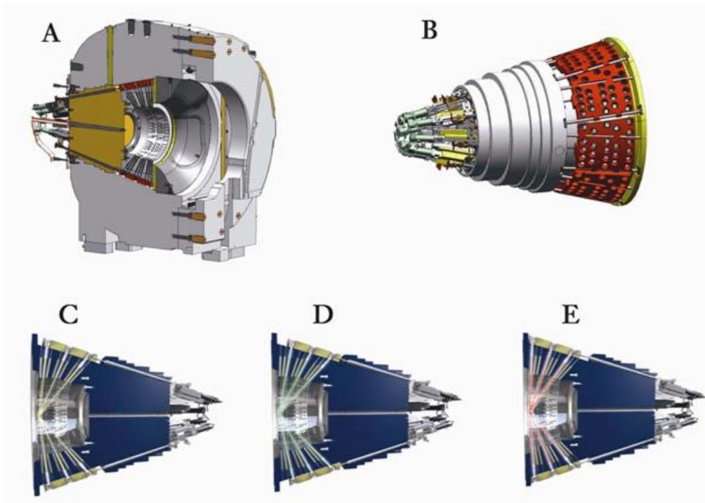
**Figure 3:** Diagrams of the PERFEXION Gamma Knife radiation unit and collimator system. A) Cross section of the Leksell Gamma Knife PERFEXION radiation unit. B) Each sector holds 24  $^{60}\text{Co}$  sources and can be moved independently on other sectors to the desired position to define collimator size or block groups of beams. C) Sector position in 4 mm collimator. D) Sector position in 8 mm collimator. E) Sector position in 16 mm collimator.
