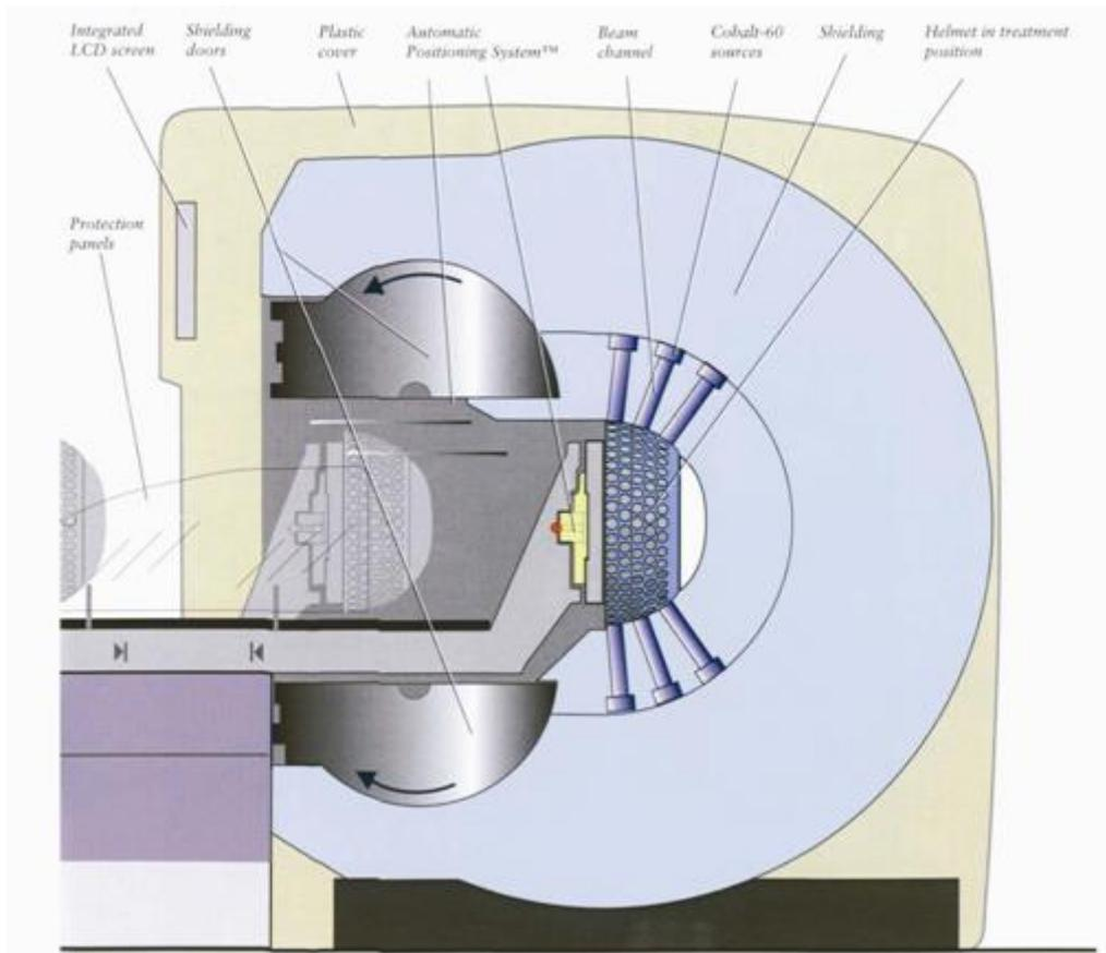
**Figure 1:** Schematic diagram of the Leksell Gamma Knife 4C
